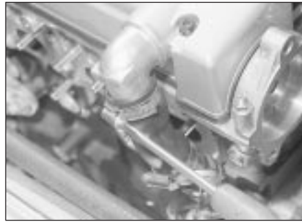
11.15 Disconnecting the large breather hose
